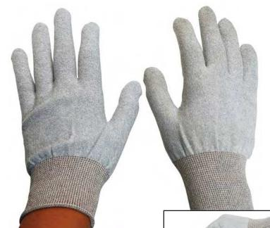
A properly grounded operator can touch a charged ESD sensitive device and a damaging ESD event can occur (Charged Device Model). Increasing the electrical path's contact resistance is one way to control the speed of the discharge and reduce the possibilities of damage. A good way to accomplish this is by wearing static dissipative gloves.
