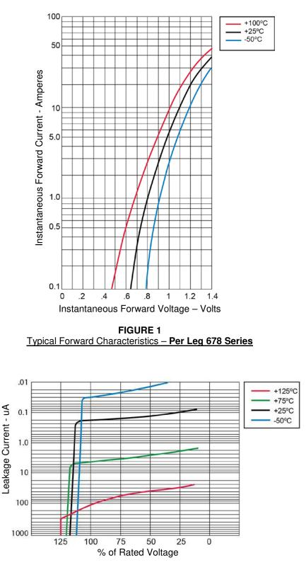
FIGURE 2 <u>Typical Reverse Leakage Current – Per Leg 678 & 682 Series</u>
