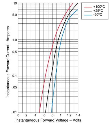
FIGURE 5 Typical Forward Characteristics – Per Leg 695 & 696 Series
