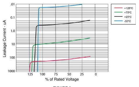
FIGURE 6 Typical Reverse Leakage Current – Per Leg 695 & 696 Series
