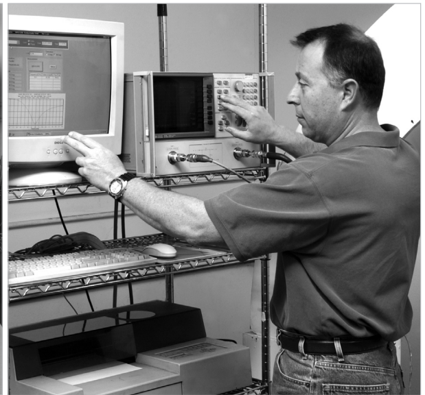
Computer controlled network analyzer provides amplitude and phase measurements on microwave absorbers.
