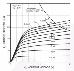
Fig. 12 Output Current vs Output Voltage (6N138M / 6N139M Only)
