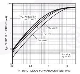
Fig. 11 Output Current vs. Input Diode Forward Current (6N138M / 6N139M Only)
