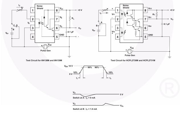
Fig. 16 Common Mode Immunity Test Circuit
