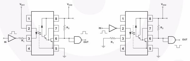
Fig. 4 Non-Inverting Logic Interface in 5 Inverting Logic in Fig. 5 Inverting Logic Interface
