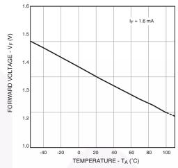
Fig. 7 LED Forward Voltage vs. Temperature
