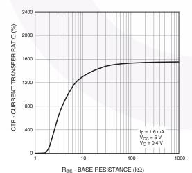
Fig. 10 Current Transfer Ratio vs. Base-Emitter Resistance (6N138M / 6N139M Only)
