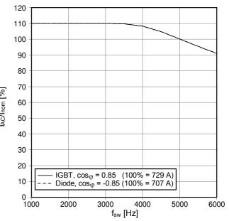
$T_{\text{inlet}}$  - derating curve IGBT (motor), Diode (generator)  $V_{DC}$  = 650 V,  $V_{AC}$  = 400  $V_{RMS},\,f_{sw}$  = 5 kHz,  $f_{AC\,\,\text{sine}}$  = 50 Hz,  $cos_{\oplus}$  =  $\pm 0.85$  and nom. cooling conditions
