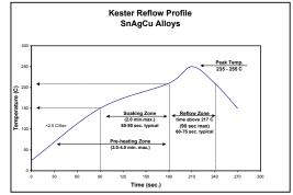
Note: TAL should be calculated based on the liquidus point of the alloy used: SAC305 221°C. Adding a soak between 180 and 200°C for 20-30 seconds can further reduce voiding and reduce the potential for tombstoning.
