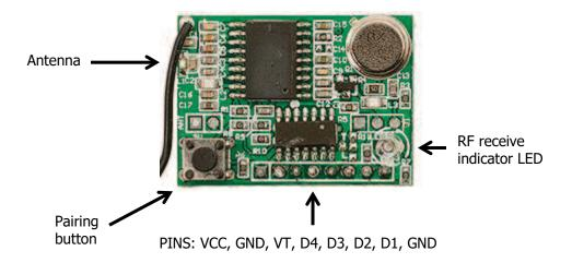
The Receiver Board has a pre-soldered antenna in "ANT2". You can uncoil the antenna to help increase the range. Typical range is ~50 feet, line-of-sight. To add even more range to the receiver you can add your own antenna to "ANT1" on the receiver board.
