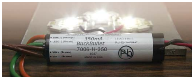
7006 BuckBullet™ LED Driver Module powering (3) Endor Star LEDs in series ( V_{IN} \geq 12VAC )
