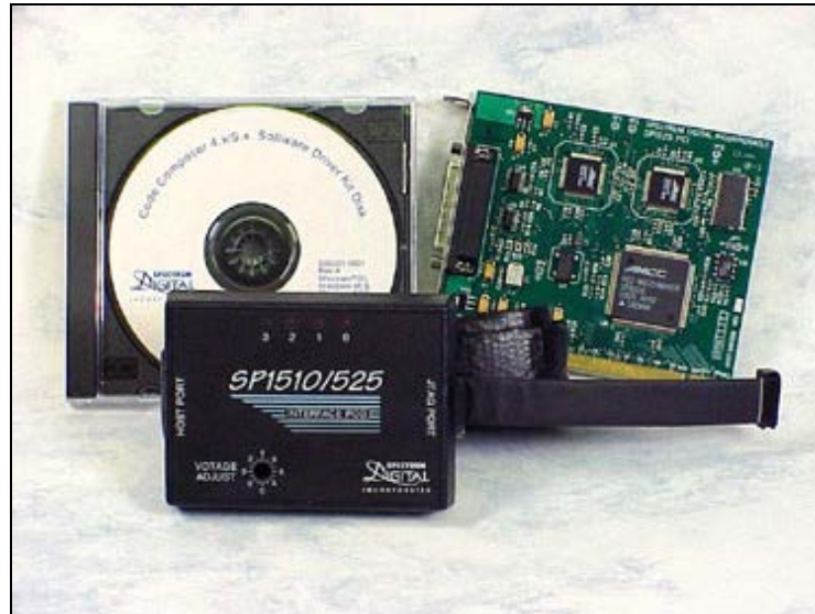
SPI510 ISA JTAG Emulator with Adjustable Voltage Pod and Code Composer for TMS320VC33/C4x
