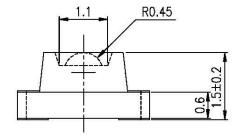
For reflow soldering (propose)
