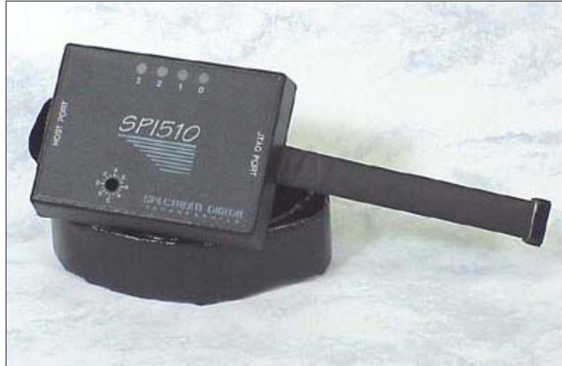
SPI510 ISA JTAG Emulator with Adjustable Voltage Pod
