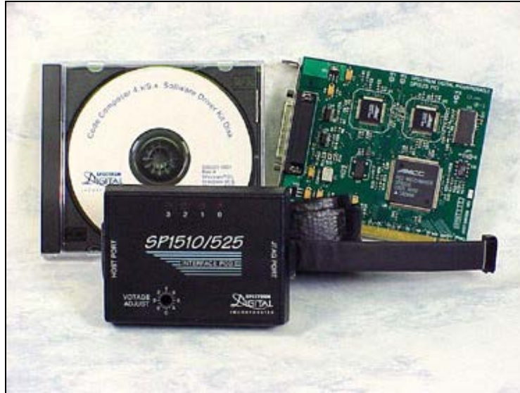
SPI525 PCI JTAG Emulator with Adjustable Voltage Pod and Code Composer for TMS320VC33/C4x
