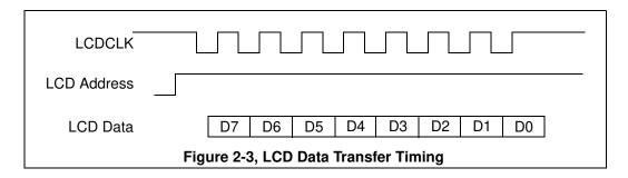
After any write operations the CPLD sets the LCD BUSY bit in the VC5502 EVM interface Register as the output is being serialized. The user should check this bit prior to starting another write operation. When LCD BUSY is high, the LCD shift register is busy, when is low the shift register is ready.
