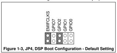
The jumpers drive signals that directly correspond to the input on one of the DSP's configuration pins. If the jumper is on, the signal is driven to a logic 0. If the jumper is off, the signal is driven to a logic 1.
