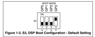
The switches drive signals that directly correspond to the input on one of the DSP's GP[3-0] configuration pins. If the switch is on, the signal is driven to a logic 0. If the DSP. A view of the switch is shown in the figure below.
