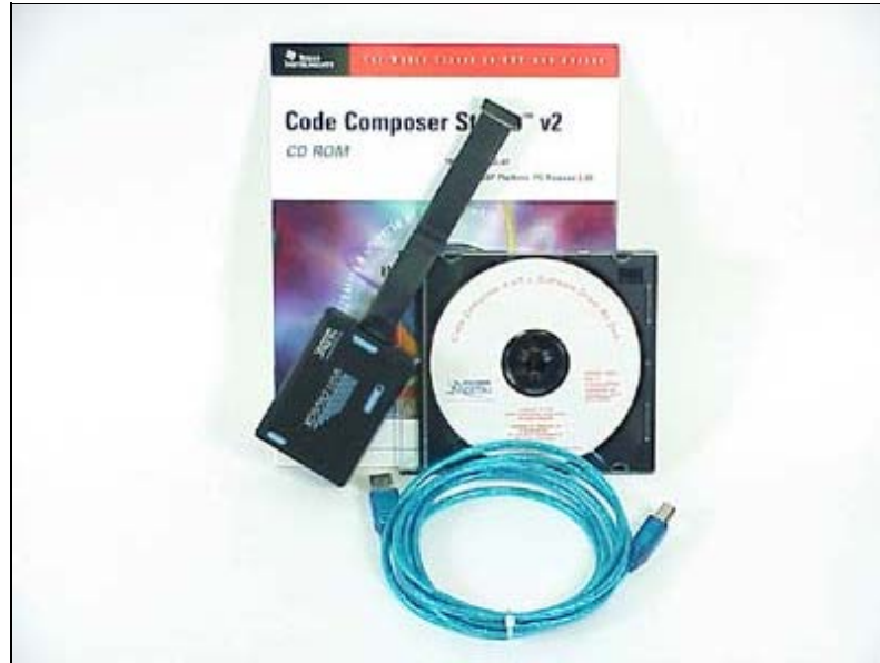
XDS510 USB JTAG Emulator with Code Composer Studio C2000 version 3.3
