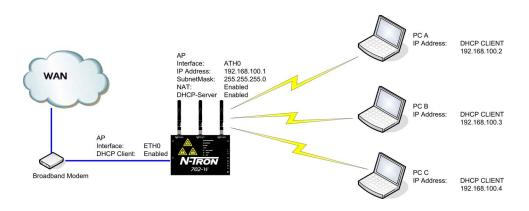
The 702-W configured as a powered router allows Layer 3 routing to setup network segmentation. It supports the Network Address Translation (Masquerading) feature which is widely used by access points. NAT will act as the firewall between LAN and WLAN networks. Additional firewall settings can be configured for Layer 3 packet filtering and access control in router mode. It can also act as a DHCP server, automating the assigning of IP addresses.
