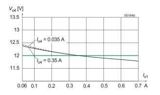
Fig. 9 Cross load regulation (typ.) on powertrain 1.  $V_{04}$  versus  $I_{01}$
