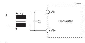
Fig. 15 External filter circuitry
