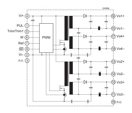
Fig. 1 Block diagram of quad-output models
