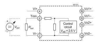
Fig. 13 Output voltage control by means of the Trim input
