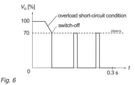
Overload switch off (hiccup mode), typical values.
