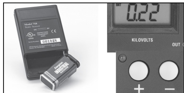
Figure 2. SCS 718 and 718A Battery Replacement and Indicators.
