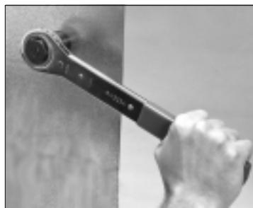
4 Turn draw stud clockwise with the 34941 wrench until material is punched.
