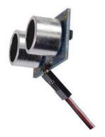
The bending of the connector assembly provides the necessary space for the two sensors to be mounted in close proximity to each other.
