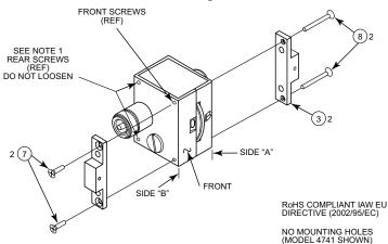
This drawing gives instructions for installation of panel mounting brackets on a model 741, 4741, 743, 4743, 745, 4745, thumbwheel turret attenuator.
