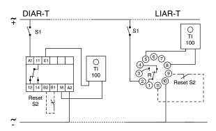
**Note:** Upon energization of the current control IAR.T Series Relay, the time delay, which is adjustable from .1 to 10 seconds, inhibits the output relay during start-up periods. The delay time is adjustable via a potentiometer located on the side of the case. For additional current transformer see "Accessories" section: L595 Series.
