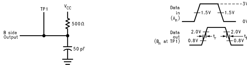
FIGURE 4. A to B Direction Test Load and Waveforms for Open Drain B 1 - B 7
