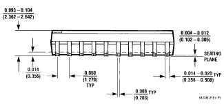
Figure 3. 20-Lead Small Outline Integrated Circuit (SOIC), JEDEC MS-013, 0.300" Wide Package Number M20B
