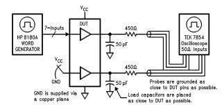
Figure 2. Simultaneous Switching Test Circuit
