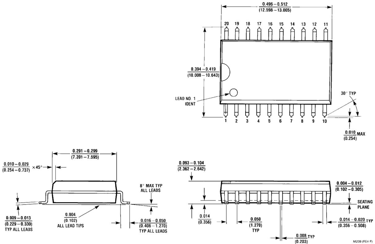
Figure 3. 20-Lead Small Outline Integrated Circuit (SOIC), JEDEC MS-013, 0.300" Wide
