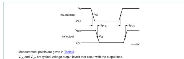
Fig 6. The input (nA, nB) to output (nY) propagation delays
