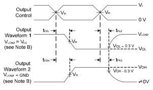
Voltage Waveform Enable and Disable Times
