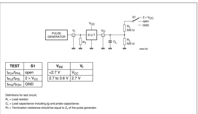
Fig.7 Load circuitry for switching times.
