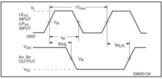
Waveform 2. Latch enable input (LEAB, LEBA) and clock pulse input ( $CP_{AB}$ ,  $CP_{BA}$ ) to output propagation delays and their pulse width
