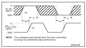
Waveform 4. Data set-up and hold times for the An and Bn inputs to the LE<sub>AB</sub>, LE<sub>BA</sub>, CP<sub>AB</sub> and CP<sub>BA</sub> inputs
