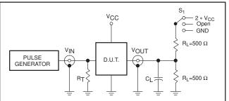
**Test Circuit for 3-State Outputs**
