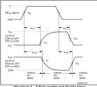
Waveform 3. 3-State enable and disable times
