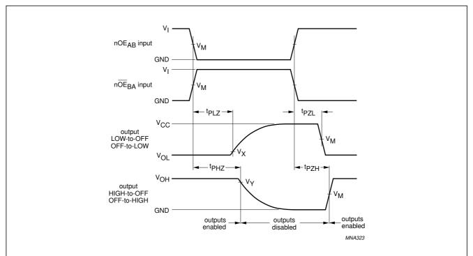
Fig.9 The OE inputs ( $nOE_{AB}$ ,  $n\overline{OE}_{BA}$ ) to outputs  $nA_n$ ,  $nB_n$  enable and disable times and the input rise and fall times.
