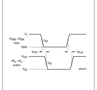
Fig.7 The inputs  $nS_{AB}$ ,  $nS_{BA}$  to outputs  $nB_n$ ,  $nA_n$  propagation delays.
