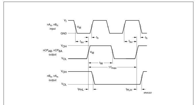
Fig.8 The nA<sub>n</sub>, nB<sub>n</sub> to nCP<sub>AB</sub>, nCP<sub>BA</sub> set-up and hold times, clock nCP<sub>AB</sub>, nCP<sub>BA</sub> pulse width, maximum clock pulse frequency and the nCP<sub>AB</sub>, nCP<sub>BA</sub> to output nB<sub>n</sub>, nA<sub>n</sub> propagation delay times.
