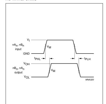
$\label{eq:Fig.6} \begin{array}{ll} \text{Fig.6} & \text{The inputs } nA_n, \, nB_n \text{ to outputs } nB_n, \, nA_n \\ & \text{propagation delay times.} \end{array}$
