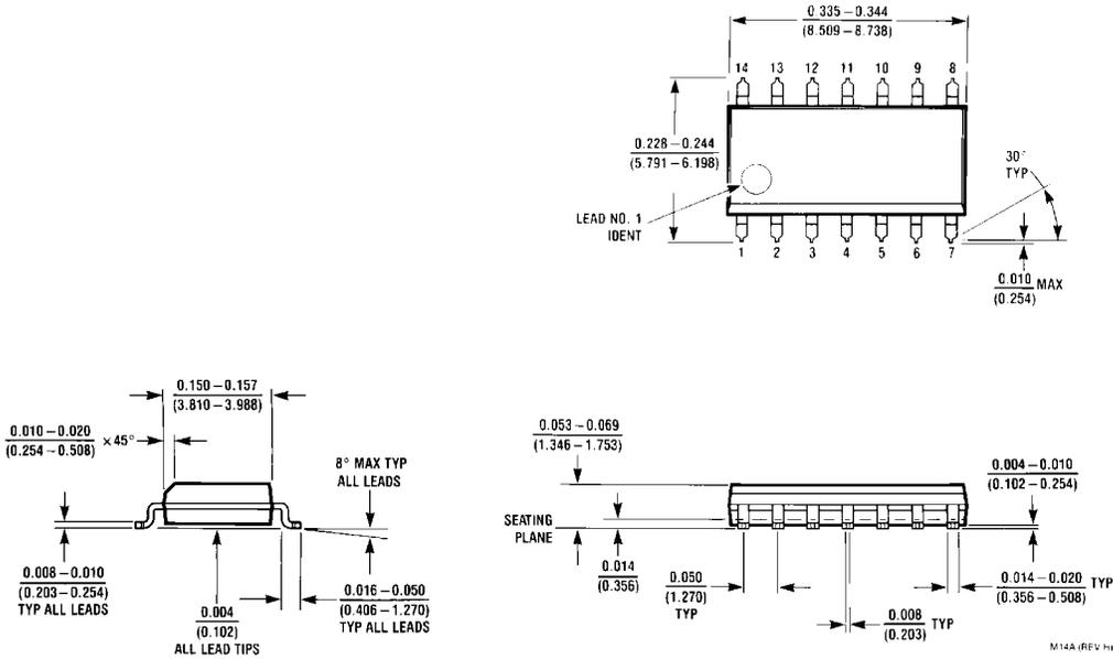
**14-Lead Small Outline Integrated Circuit (SOIC), JEDEC MS-120, 0.150 Narrow
