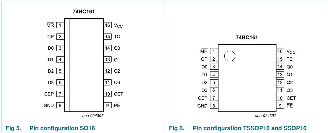
Fig 5. Pin configuration SO16
