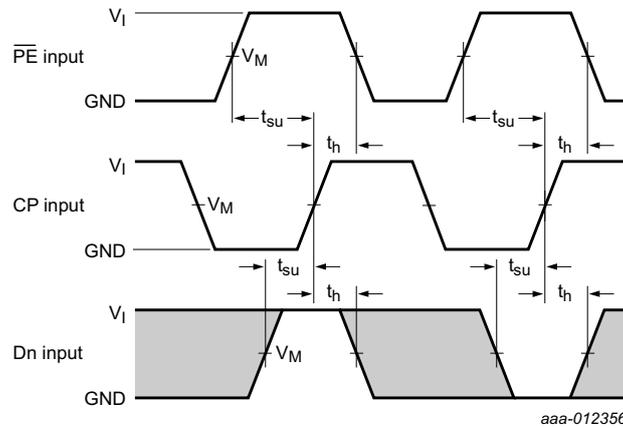
The shaded areas indicate when the input is permitted to change for predictable output performance. Measurement points are given in [Table 8](#).
