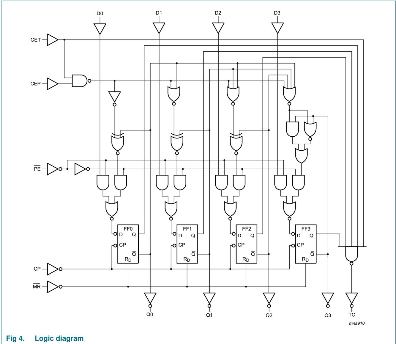
Fig 4. Logic diagram
