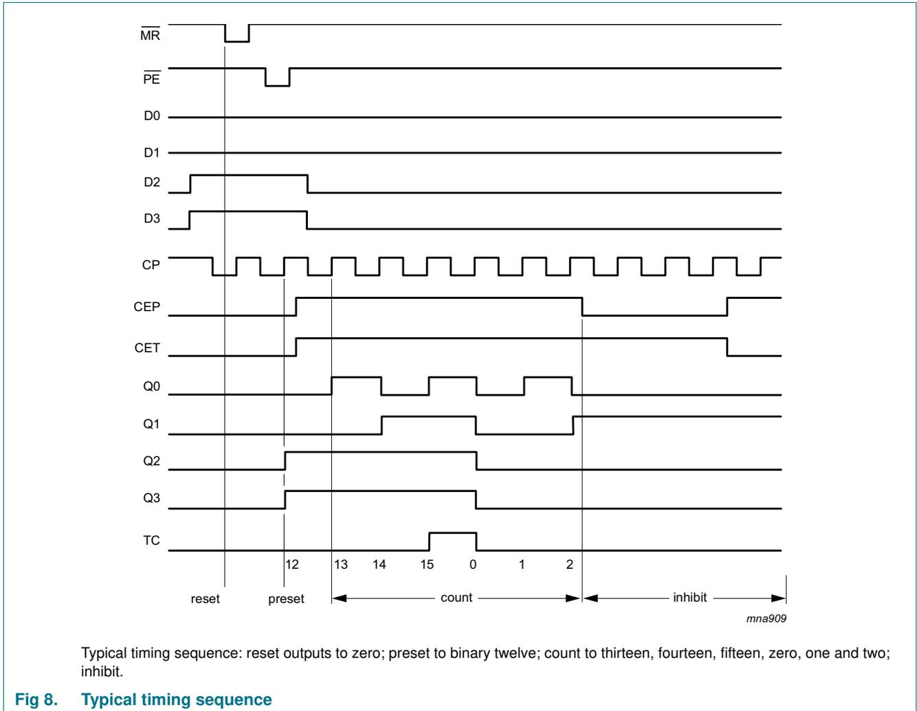
Fig 8. Typical timing sequence
