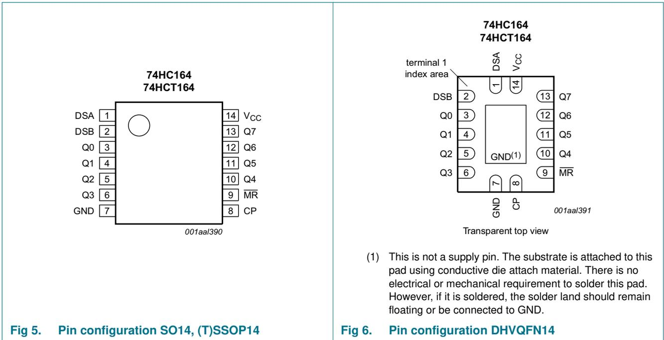
Fig 5. Pin configuration SO14, (T)SSOP14
