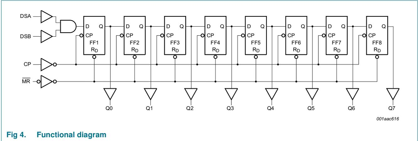
Fig 4. Functional diagram
