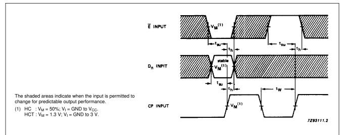
Fig.7 Waveforms showing the data set-up and hold times from the data input  $(D_n)$  and from the data enable input  $(\overline{E})$  to the clock (CP).
