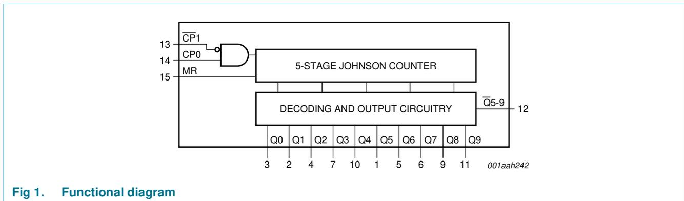
Fig 1. Functional diagram
