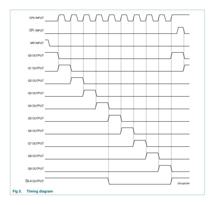
Johnson decade counter with 10 decoded outputs
