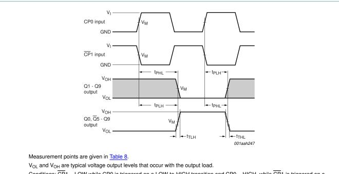
Conditions:  $\overline{CP1}$  = LOW while CP0 is triggered on a LOW-to-HIGH transition and CP0 = HIGH, while  $\overline{CP1}$  is triggered on a HIGH-to-LOW transition.
