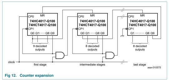
**Remark:** Do not enable the counter on  $\overline{CP1}$  when CP0 is HIGH, or on CP0 when  $\overline{CP1}$  is LOW. It causes an extra count.
