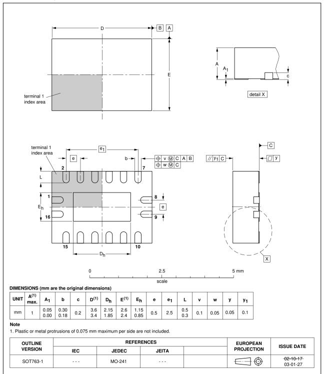
DHVQFN16: plastic dual in-line compatible thermal enhanced very thin quad flat package; no leads; 16 terminals; body 2.5 x 3.5 x 0.85 mm SOT763-1
