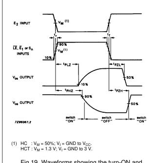
Fig.19 Waveforms showing the turn-ON and turn-OFF times.
