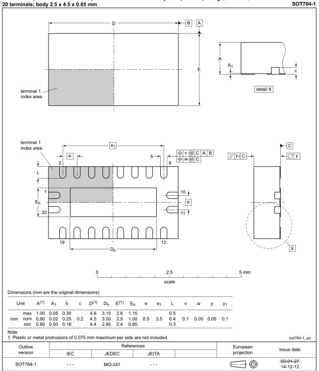
DHVQFN20: plastic dual in-line compatible thermal enhanced very thin quad flat package; no leads; 20 terminals: body 2.5 x 4.5 x 0.85 mm
