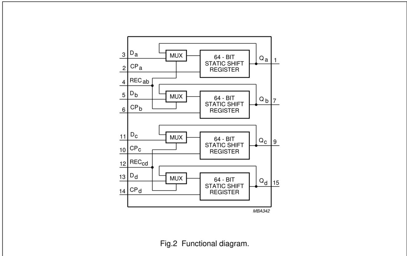
Quad 64-bit static shift register
