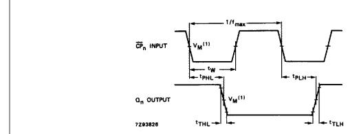
(1) HC :  $V_M$  = 50%;  $V_I$  = GND to  $V_{CC}$ . HCT:  $V_M$  = 1.3 V;  $V_I$  = GND to 3 V.
