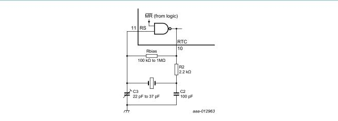
Fig 17. External components connection for a typical crystal oscillator
