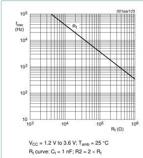
Fig 15. RC oscillator frequency as a function of Rt
