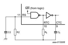
Typical formula for oscillator frequency:  $f_{osc} = \frac{1}{2.5 \times R_t \times C_t}$
