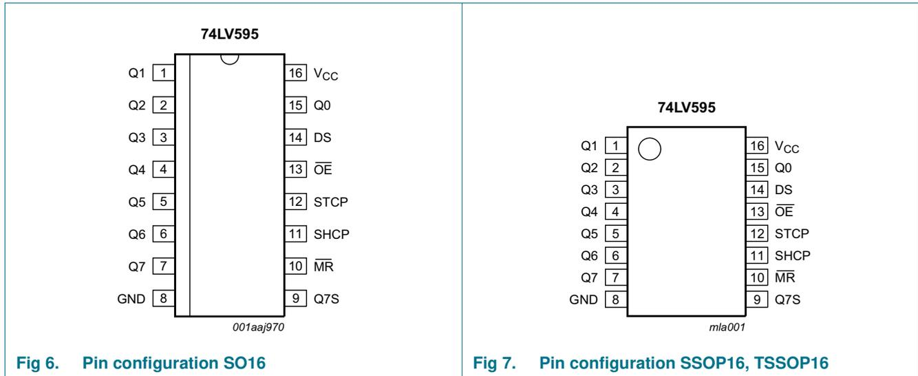
Fig 6. Pin configuration SO16
