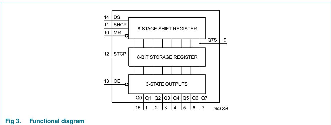
Fig 3. Functional diagram
