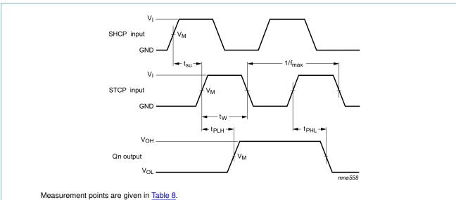
V<sub>OL</sub> and V<sub>OH</sub> are typical output voltage drops that occur with the output load.
