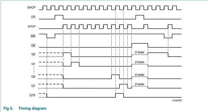
8-bit serial-in/serial-out or parallel-out shift register; 3-state
