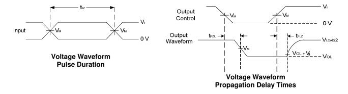
Notes: A. Includes test lead and test apparatus capacitance. B. All pulses are supplied at pulse repetition rate  $\leq$  10 MHz
