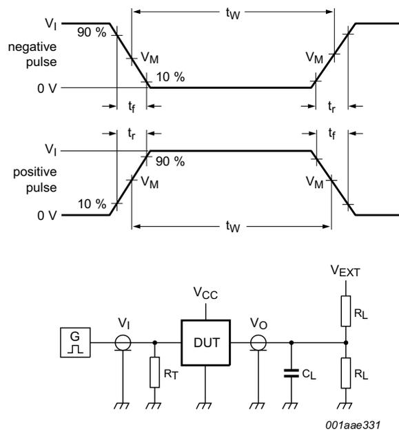
Test data is given in [Table 9](#). Definitions for test circuit:
