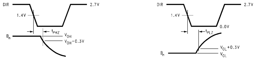
FIGURE 6. t_{PHZ} and t_{PLZ} Test Load and Waveforms DIR to B_1-B_8
