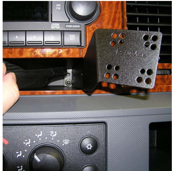
InDash Installed Showing Screws in Place
