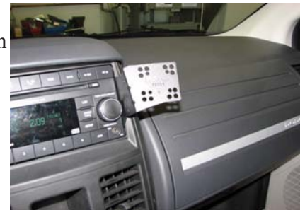
Mount installed on 08-10
