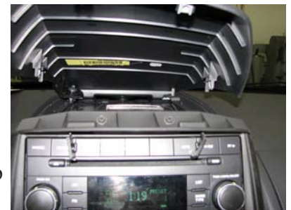
Cover Removal and screws under cover
