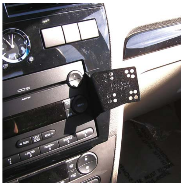
InDash installed showing location on Right Side
