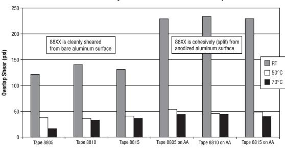
3M™ Thermally Conductive Adhesive Transfer Tapes
